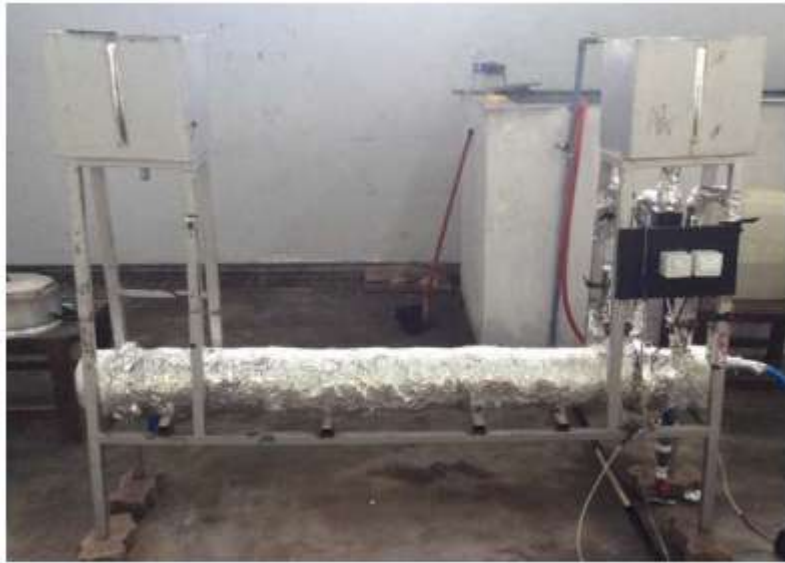
Gambar 5 Proses Pengujian Heat Exchanger
